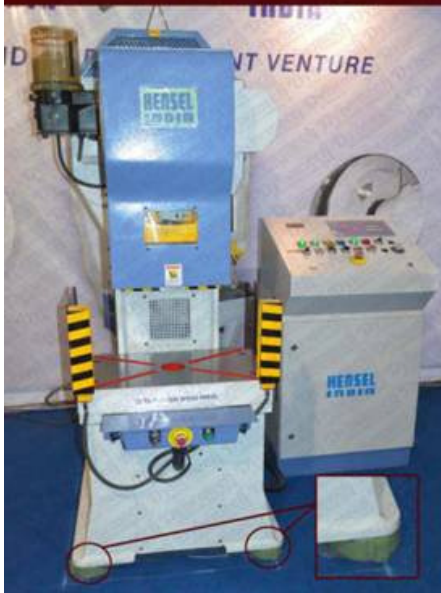
Fig 4: Large Power Presses on Dynemtech Wedge Mounts & Screw Support Vibro-Mounts
