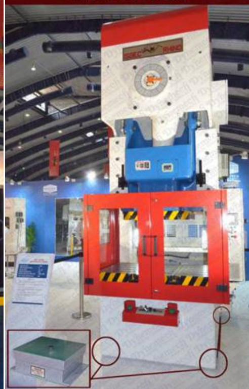
Fig 1: Power Presses on Dynemtech Spring Isolators & Wedge Mounts
