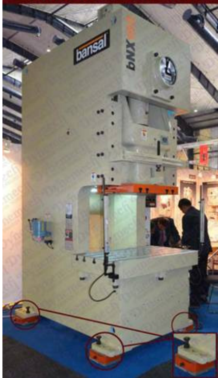
Fig 1: Power Presses on Dynemtech Spring Isolators & Wedge Mounts
