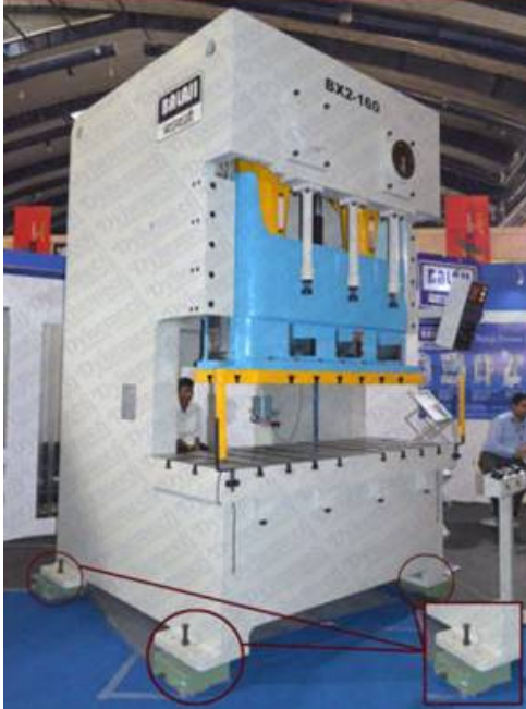
Fig 3: Power Presses on Dynemtech Spring Isolators & Wedge Mounts
