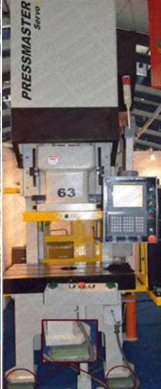
Fig 1: Power Presses on Dynemtech Spring Isolators & Wedge Mounts
