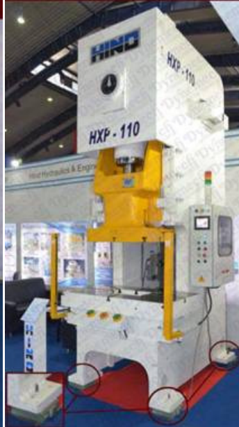
Fig 4: Large Power Presses on Dynemtech Wedge Mounts & Screw Support Vibro-Mounts
