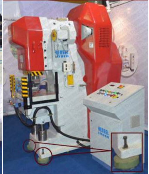
Fig 4: Large Power Presses on Dynemtech Wedge Mounts & Screw Support Vibro-Mounts
