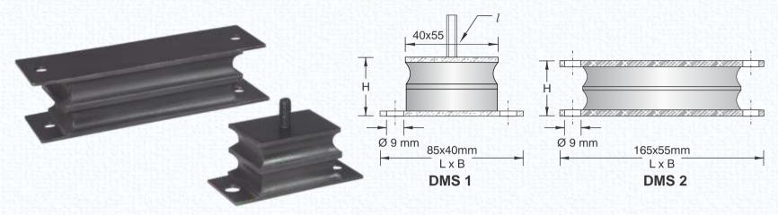
The Sandwich mounts comprise one or more layers of elastomer bonded to flat steel plates. They are designed to withstand very high compressive loads. They are very slim, large supporting surface area, stackable mounts. The suspended equipment is free to move in all directions. High ratio of axial stiffness to radial stiffness. Very high axial loads.
